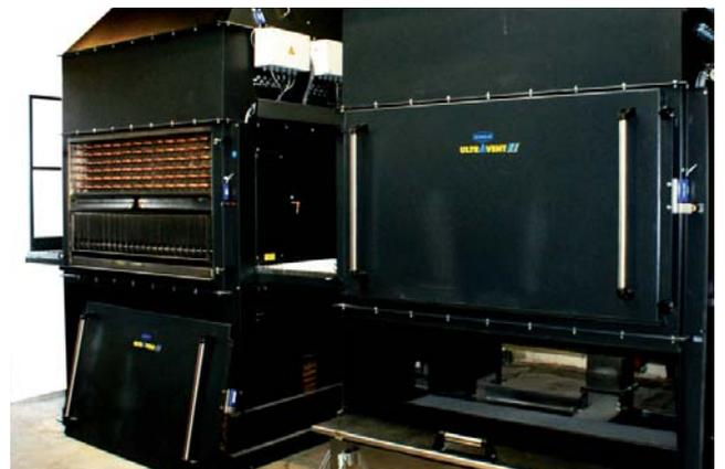
Pict.: ULTRAVENT® air filter with demister, electrostatic precipitator and heat exchanger (from the bottom upwards). The automatic filter cleaning system is placed between the electrostatic filter and heat exchanger module.
