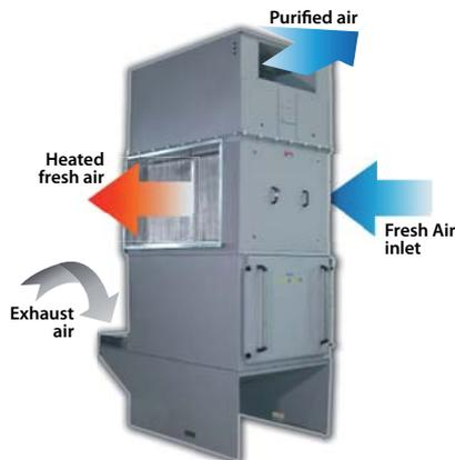
Cool air from outdoors is directed horizontally through the device and is heated up. Both air flows have to be led through the heat exchanger in a counter current way. Thereby the incoming air and the exhaust air are separated by a heat-conducting surface, so the two cannot be mixed with each other
