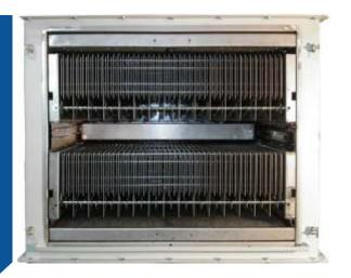
4) Low maintenance by automatic cleaning system (CIP)
